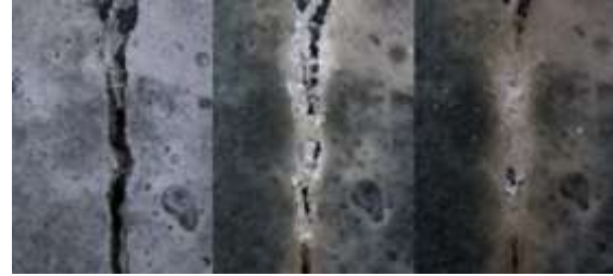
Figure 1: Sealing of Cracks with calcium carbonate crystals
